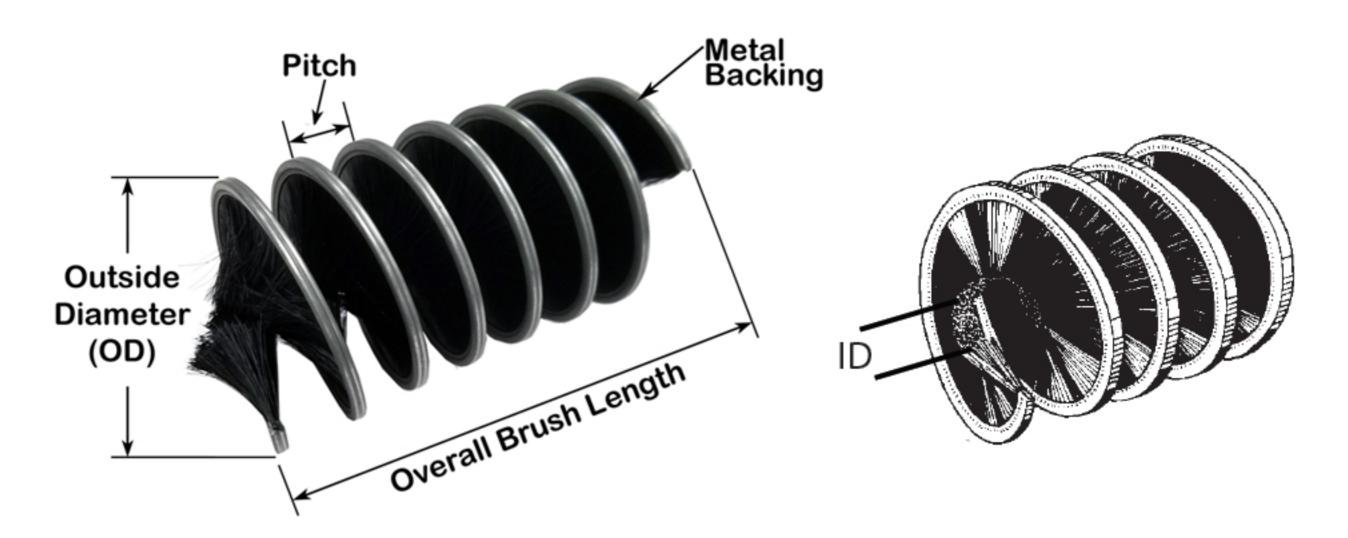
Inward Wound Coil Brushes are made from a Metal Backing (Channel) Strip brush that is formed into a "Coil or Spiral" shape.
